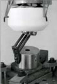
Set-up for biomechanical Targon FN lab testing
